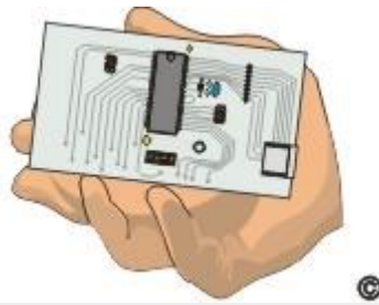
Figure 1: Always handle circuit boards by the edges.
